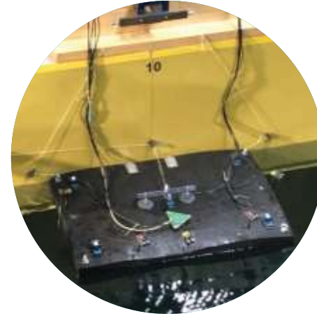
Softshell, Mass Evacuation System (MES) model - Neoprene foam
